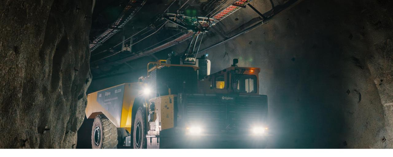
Boliden, Epiroc and ABB make first battery-electric truck trolley system for underground mining a reality
