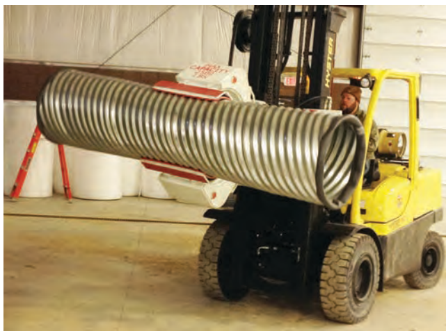
Empty J-PAK shell being moved.
