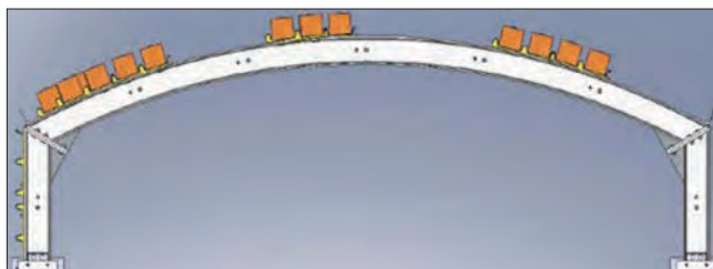
Impact Resistant Arch Set Design for Roof Fall Rehabilitation
