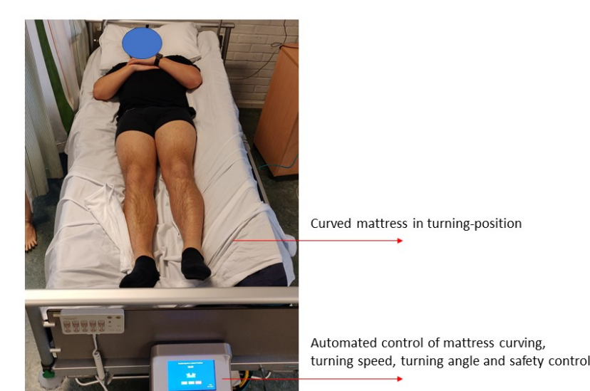
Figure 2. The test set-up consisted of an ordinary rubber foam mattress that is placed on top of the innovative mattress system. A pressure imaging sensor mat was placed on top of the rubber foam mattress.
