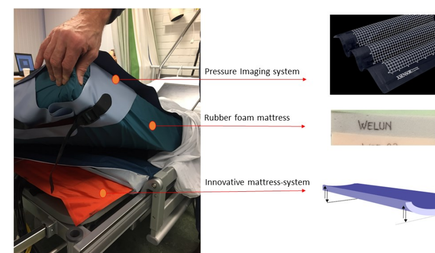
Figure 2. The test set-up consisted of an ordinary rubber foam mattress that is placed on top of the innovative mattress system. A pressure imaging sensor mat was placed on top of the rubber foam mattress.
