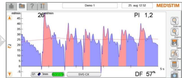
After revision (proximal anastomosis corrected) High flow, low PI, normal DF and regular curves
